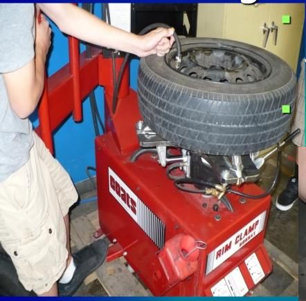
Remove hose and **QUICKLY** install the core into the valve stem. Check & Adjust Pressure as
