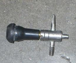
Using a Tire Stem Core-Removal Tool
