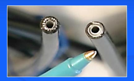
notice the plastic liner inside the housing – this is what the cable slides back and forth on – no lubrication needed!
