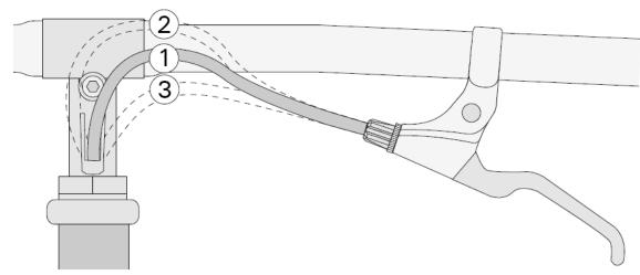
**35.6** When the housing length is correct, it enters the stop below the stem in a straight line (1). When the housing length is too long (2) or too short (3), the housing enters the stop below the stem or at the brake at an angle.
