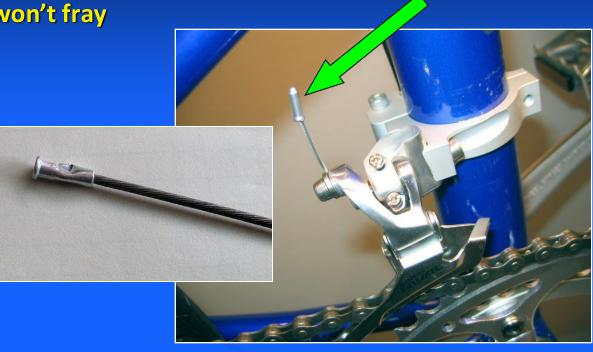
DO NOT cut the cable or install the cable cap until you test ride your bike and you are satisfied brakes and shifters work properly!!!
