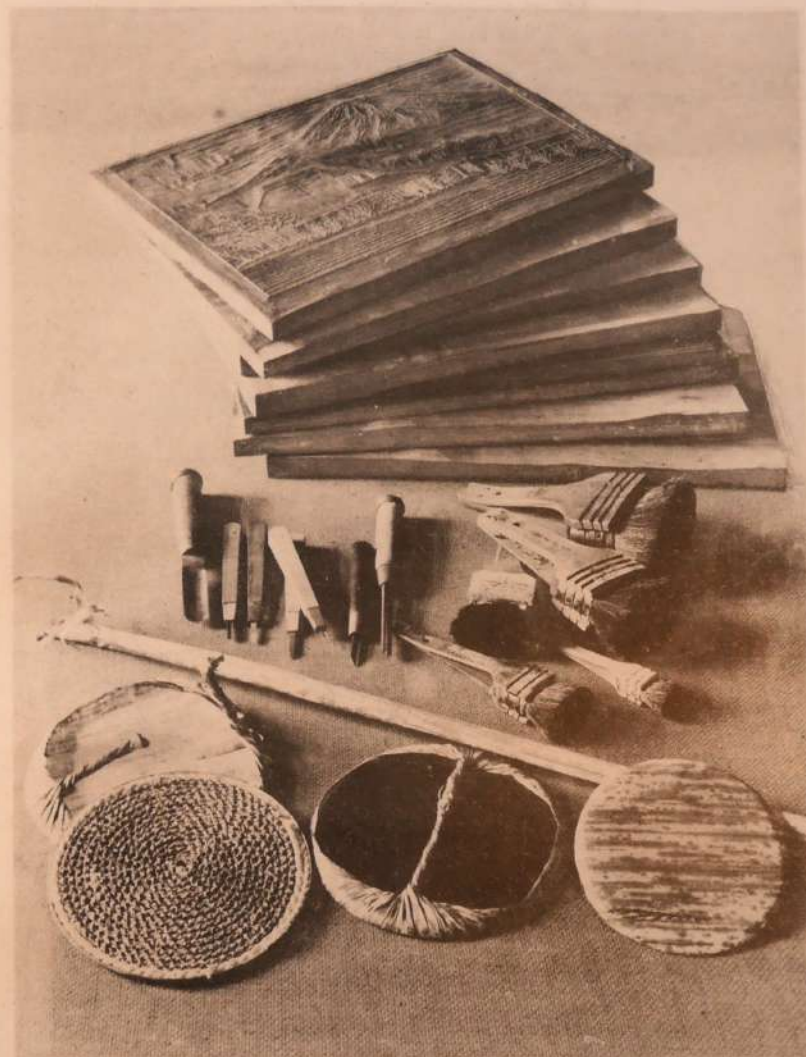
On top is a set of printing wooden blocks, each of which is carved on both sides. Since there are seven blocks, it means that no less than fourteen impressions are required to make a print in this case. In the middle are a knife, chisels and paint-brushes used in carving and colouring. At bottom are a barén , or press pad, (middle), parts thereof and its bamboo sheath material. On the left is a bamboo-sheath basket into which is inserted a plaited mat of bamboo sheath threads and over it is fixed a disc (bottom white and top black) made of fifty-five sheets of thin paper pasted together. On the extreme right is shown the rubbing side of the barén . Great skill is needed to make a barén and years' training is necessary to produce a proper barén .
